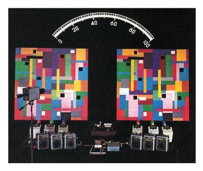
In a typical experiment, the illuminators were adjusted so that an area of the Mondrian at the left and some differently-colored area of the Mondrian at the right were both sending the same triplet of radiant energies to the eye. In the example below, the eye perceives the exact same triplet of long-, middle-, and short-wave energies from the red area (left) and the blue area (right).
